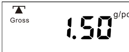
Press %/◀ key again to check the total weight of the sample. ("s" indicates that the scale is in counting mode)
