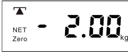
Press **TARE/▲** key to eliminate the preset tare value when the display shows as above.
