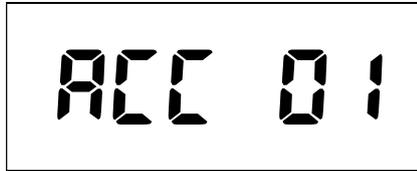
2 seconds later, the display shows the accumulated sample weight.
