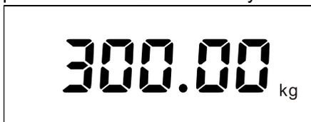
A few seconds later, the buzzer sounds, and the scale counts backwards to zero. The calibration procedure is finished. Then switch off and take away all the weights.
