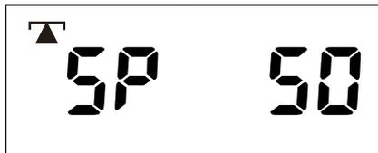
After you have chosen the sample size, put on the sample with a quantity the same as the sample size you have chosen. Then press **ZERO/ENTER** key & the display shows "-----"; several seconds
