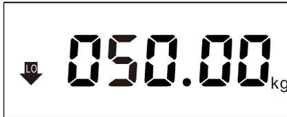
Press **ZERO/ENTER** key to confirm the value you have set. Then the scale returns to normal weighing mode.
