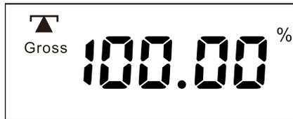
Take off the sample, and put on the objects to be measured, then the display will show a percentage (the current weight to the sample weight)
