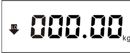
Press **TARE/▲** key to change the value of the flashing digit; press **Check-W/▶** and **%/◀** key to move the flashing digit to right or left.
