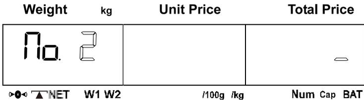
The flashing number in Weight display window indicates the current editing interface.
