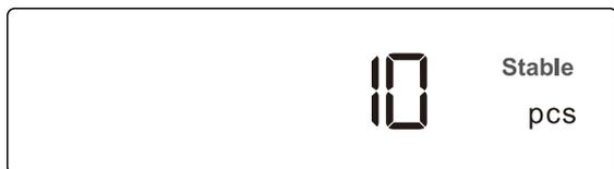
Take off the samples on the pan. The sampling operation is finished. Then the balance can be used for counting.
