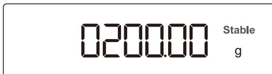
After the weight value has been set, press **ENTER** key and the value starts flickering. Then put on the mass which is the same weight as the display showing. When the display is stable, it will count down to zero automatically. Take off the mass. The calibration is finished.
